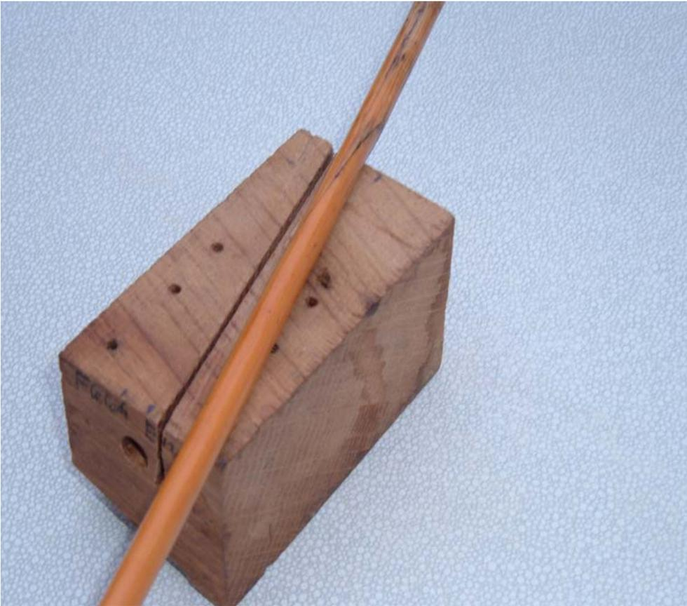
Arrow joining jig with arrow showing angle of cut.
